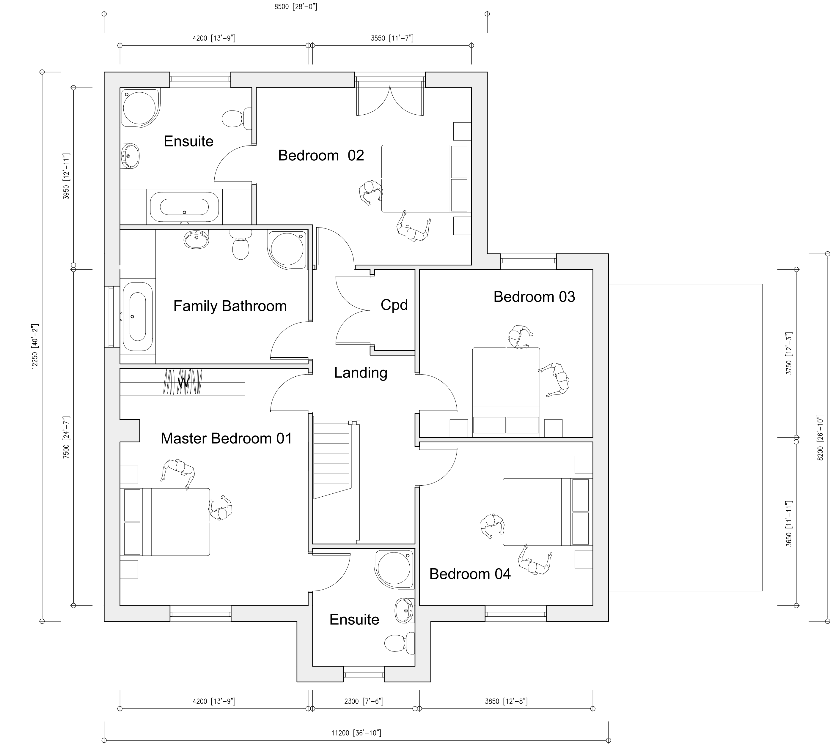
PROPOSED FIRST FLOOR PLAN SCALE 1:50
